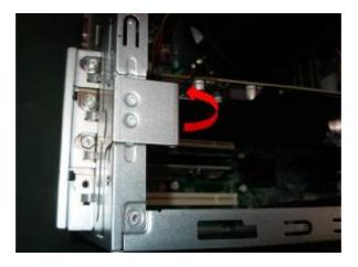
3.2 Disconnect the screw fixed in the bracket
